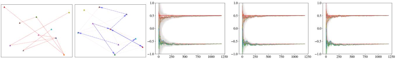
Fig. 1: Cooperative localization in a ten-agent time-varying network. Left to right: observation network, communication network at  $t = 2$ , estimates of agent 2's position for  $\alpha \in \{0.5, 1, 1.5\}$  over 1250 iterations. The horizontal red lines indicate the true position of agent 2.
