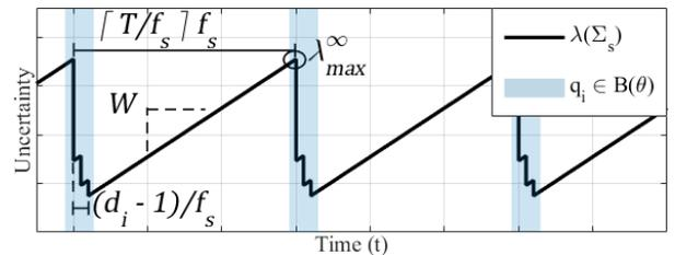
Fig. 3. Example uncertainty of Kalman filter estimate for one point with a cycle time of  $T$ ,  $d_i$  observations, and covariance of the environmental process  $\mathbf{W}$ . The shaded regions indicate when the point of interest  $q_i$  is within sensing range  $B(\theta)$ . The maximum steady-state value of the uncertainty  $\lambda_{max}^\infty$  immediately precedes the first observation.
