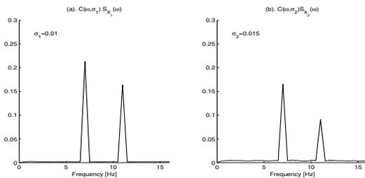
Figure 1: Power spectrum estimation of data subject to sampling jitters. (a)  $C(\omega, \sigma)S_{X_1}(\omega)$  and  $\delta_{1n} \sim N(0, \sigma=0.01)$  and (b)  $C(\omega, \sigma)S_{X_2}(\omega)$  with  $\delta_{2n} \sim N(0, \sigma=0.015)$ .
