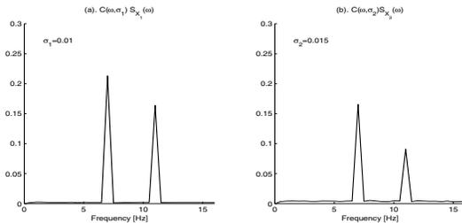
Figure 1: Power spectrum estimation of data subject to sampling jitters. (a)  $C(\omega, \sigma)S_{X_1}(\omega)$  and  $\delta_{1n} \sim N(0, \sigma=0.01)$  and (b)  $C(\omega, \sigma)S_{X_2}(\omega)$  with  $\delta_{2n} \sim N(0, \sigma=0.01)$ .
