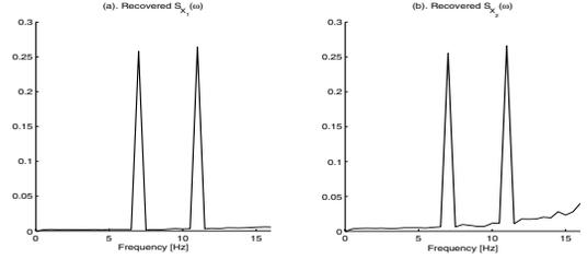
Figure 2: Restored power spectrum estimation of data subject to sampling jitters, (a)  $S_{X_1}(\omega)$  and (b)  $S_{X_2}(\omega)$ .
