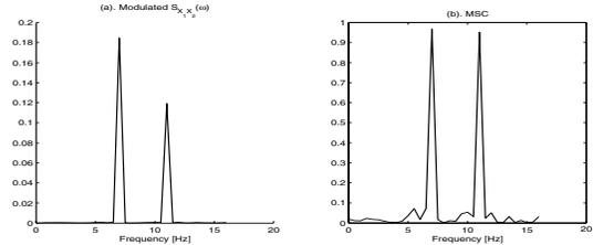
Figure 3: Estimation of dual-channel (a) Modulated Cross-Spectrum  $S_{X_1 X_2}(\omega)$ , and (b)  $MSC(\omega)$ .
