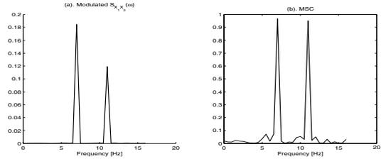
Figure 3: Estimation of dual-channel (a) Modulated Cross-Spectrum  $S_{X_1 X_2}(\omega)$ , and (b)  $MSC(\omega)$ .
