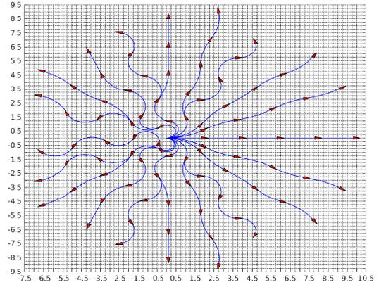
Fig. 2: The set of motion primitives used for LTL-constrained A\* planning. Each segment contains 5 robot poses indicated by the red triangles. Each robot pose represents a different motion primitive.
