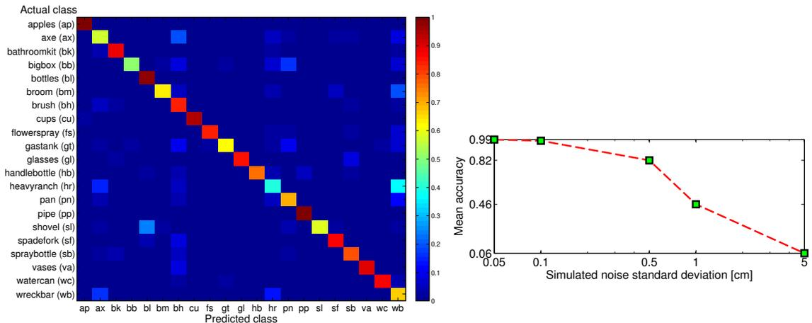
Figure 4.5: Confusion matrix (left) for all classes in the VP-Tree. A class is formed from all views associated with an object. The effect of signal noise on the classification accuracy of the VP-Tree is shown on the right.
