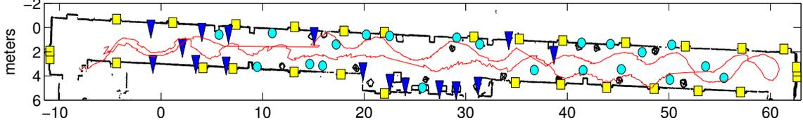
Figure 3.17: Tango phone trajectory (red) estimated via semantic localization in a real experiment. The semantic map contains doors (yellow squares), red chairs (cyan circles), and brown chairs (blue triangles). Ground-truth information was not available for this experiment. See Appendix D.16 Extension 4 for more details.
