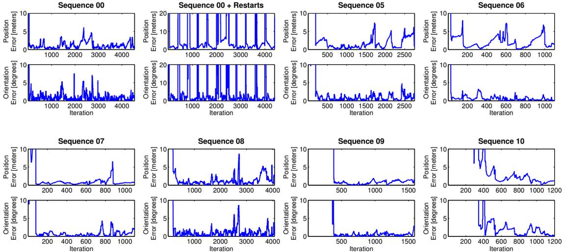
Figure 3.19: Position (euclidean distance) and orientation errors of the vehicle trajectories recovered via global semantic localization on sequences  $\{00, 05, 06, 07, 08, 09, 10\}$  from the KITTI visual odometry dataset. The plot, titled “Sequence 00 + Restarts”, shows results from an experiment in which the localization was restarted every 400 iterations. Appendix D.16 Extensions 5 - 13 provide videos of all experiments.
