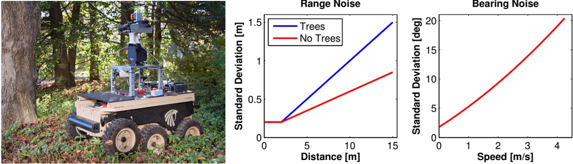
Figure 2.5: The Landshark differential-drive robot (left) tracks a mobile target through a wooded area via range and bearing measurements. The plots on the right show the dependence of the sensor performance on the robot speed, the distance to the target, and the target visibility, which can be obstructed by trees.
