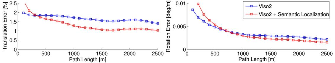
Figure 3.20: Average translation and orientation errors<sup>8</sup> obtained from visual odometry via Viso2 (Geiger et al. 2011) and from visual odometry combined with semantic localization on sequences  $\{00, 05, 06, 07, 08, 09, 10\}$  from the KITTI visual odometry dataset. Both methods use a known starting vehicle pose, i.e., perform tracking instead of global localization.
