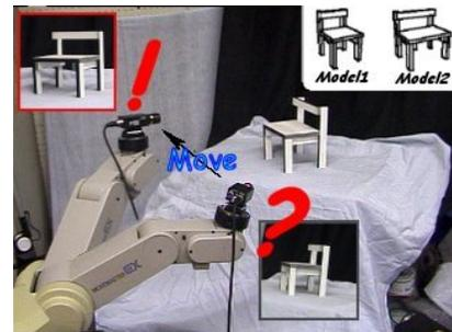
Figure 1.6: Planning the viewpoint of an autonomous camera in order to improve the results of object recognition
