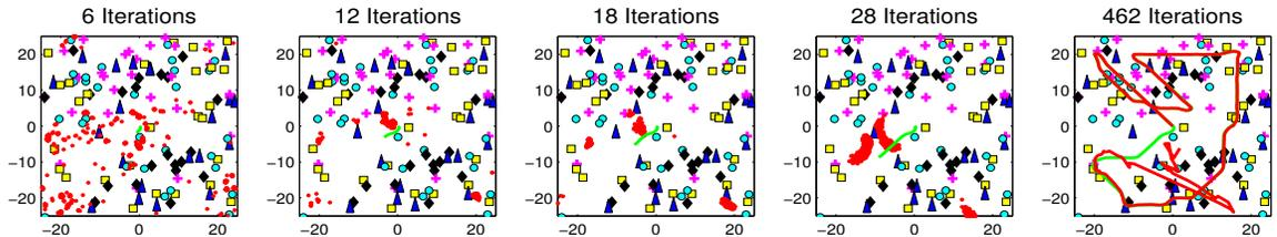
Figure 3.12: A simulated environment with 150 objects from 5 classes (circles, squares, triangles, crosses, and diamonds) in a  $25 \times 25 m^2$  area. The plots show the particles (red dots), the ground truth trajectory (green), and the estimated trajectory (red) for clutter rate  $\lambda = 4$ .
