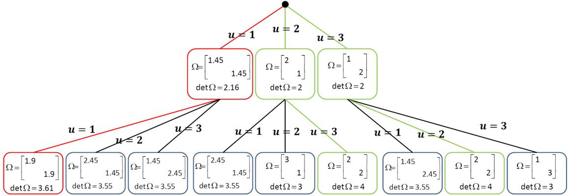
Figure 2.2: Example that greedy planning is worse than nonmyopic planning even for static independent targets and a planning horizon of  $T = 2$ . The control sequence chosen by greedy planning is indicated in red, while the optimal two-step sequences are shown in green.
