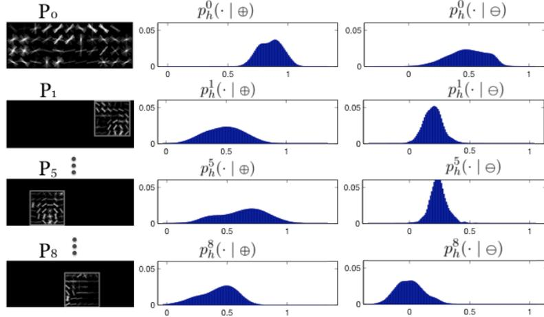
Figure 4.9: Observation models for several part filters from a car DPM. The root ( $P_0$ ) and three parts of the model are shown on the left. The corresponding positive and negative score likelihoods are shown on the right.
