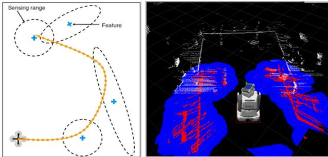
Figure 1.5: A robot can improve its localization and environment map by planning an informative trajectory for its future observations (courtesy of Vitus et al. 2012)
