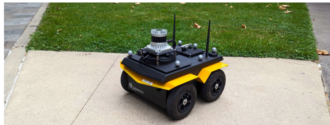
Fig. 1: Clearpath Jackal robot equipped with a LiDAR.
